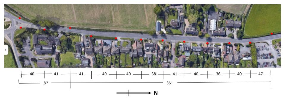
The red dots on the above plan show the location of, and distances in meters between, the lamp posts on the A5127 Shenstone Woodend from Blake Street Island to the Toby Carvery. The measurements were made using a trundle wheel and are within 1m tolerance.
